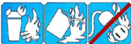
The new style of labeling shows that an extinguisher with this label (before red line) may be used on ordinary combustibles, Flammable Liquids, or electrical equipment fires. The new labeling style with a diagonal red line drawn through the picture indicates what type of fire extinguisher shall **NOT** be suitable for. In this example, fire extinguisher could be used on ordinary combustibles and flammable liquids fires, but not for an electrical equipment fire.
