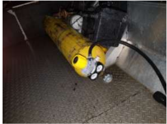
Regulator frosting up during dive at the Cedar Wapsi (C-57) Bridge _200608
